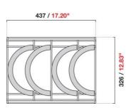
The cooling packs must be inserted vertically into the shape-maintainer rack, so that the liquid freezes in the bottom, leaving the top air chamber.
